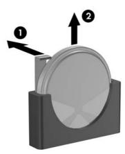
Figure 2-6 Removing and replacing the internal battery
